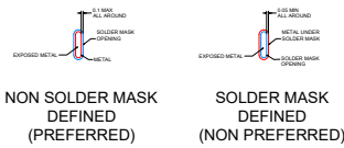
LAND PATTERN EXAMPLE EXPOSED METAL SHOWN
